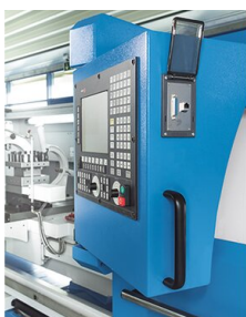
Interface for data transmission, swivelling control operating unit
